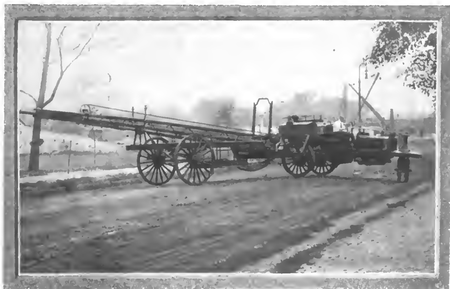
Water tower, with Martin tractor in front, recently built by the Knox company for the Springfield, Mass., fire department
